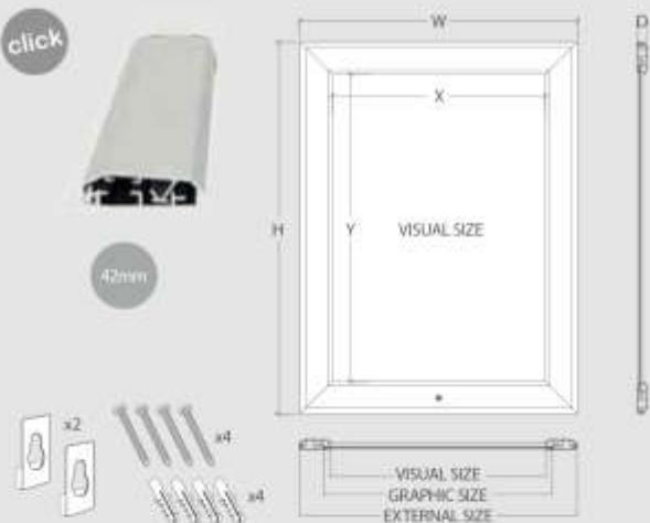
The LIMA frame is constructed from anodized aluminum with a matte silver finish and it features a front-loading frame which can be secured shut with an Allen key to keep posters protected. It can be mounted vertically or horizontally. Screws and allen key wrench included. This frame is perfect for being used in restaurants, retail stores, community centers, movie theaters, airports, banks or any other location requiring frequent changes of advertisements.
